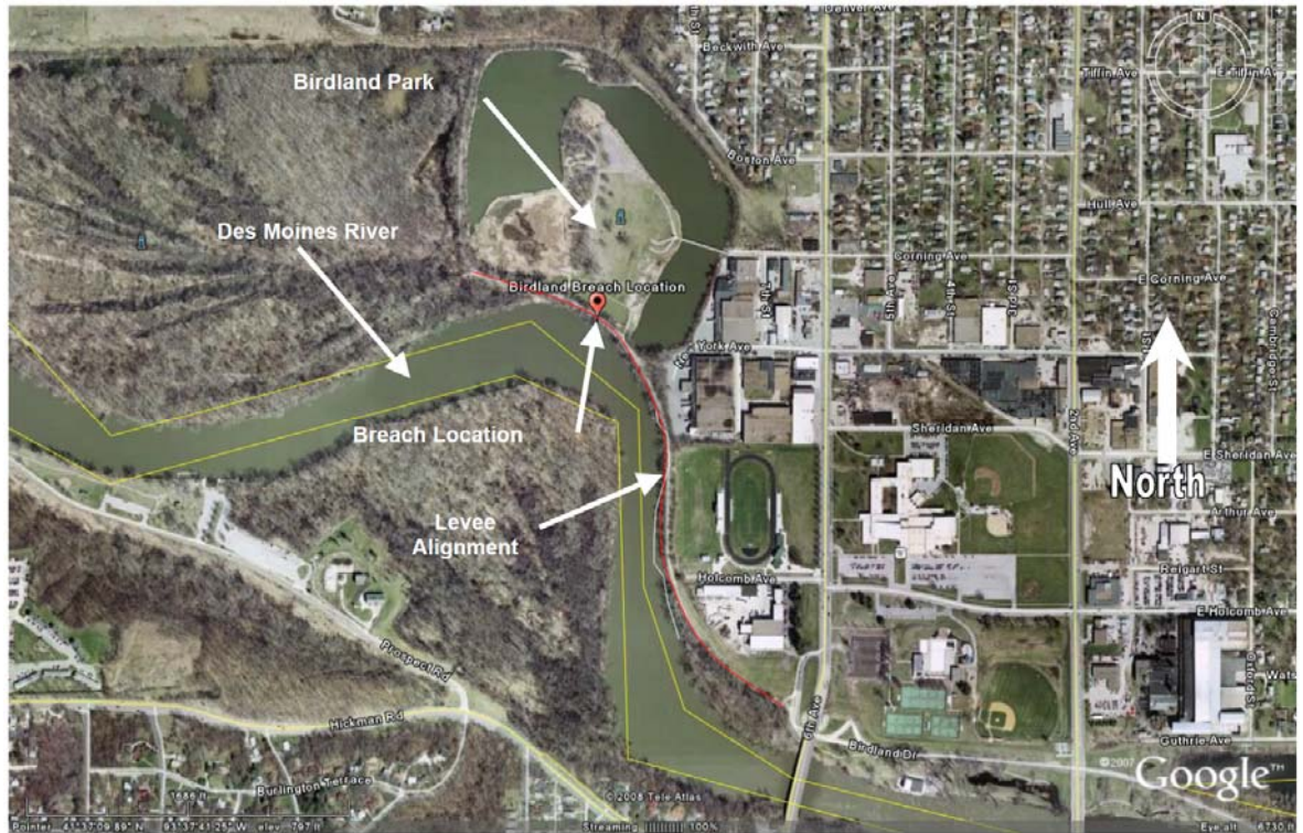
Figure 3.17 Location of the Birdland Levee breach (taken 2007).
