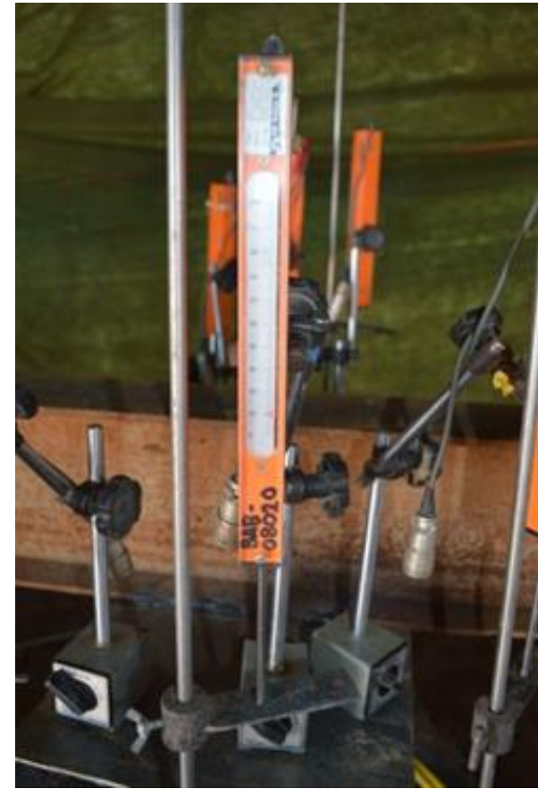
Bi-Directional static load test in construction site
