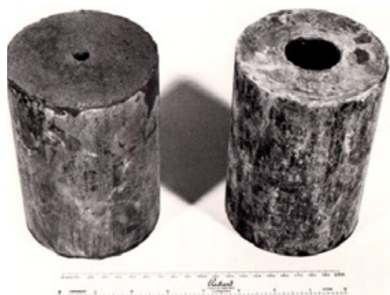
Figure 5: Test specimens for small scale pressuremeter tests in a triaxial cell
