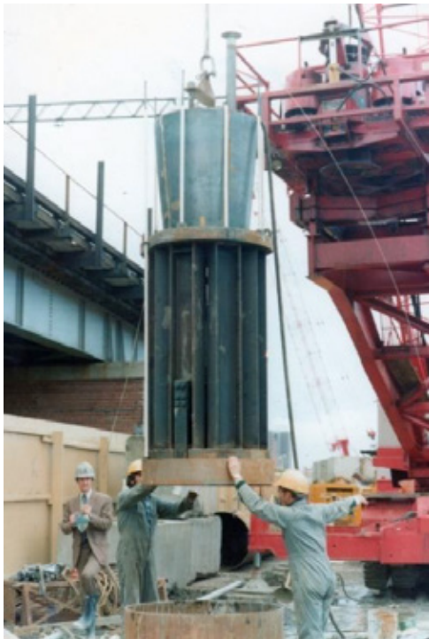
Figure 2: MURLA test rig for simultaneous base and side testing being lowered into a socket
