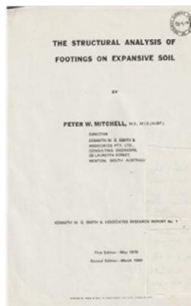
Figure 2: Title page of K W G Smith & Associates Research Report No 1 by P W Mitchell. This report described the "Mitchell Method" for design of footings for houses on reactive soil
