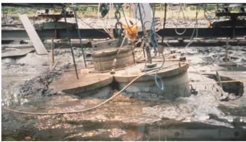
Figure 19.6. TLP model after being loaded to failure (Photo: R. Dyvik, NGI).
