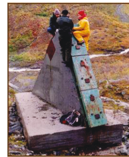
Fig. 3. Test structure with 3 load plates to measure impact forces during an avalanche (1982)
