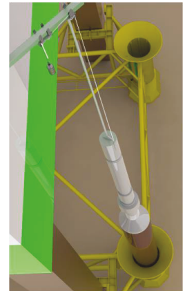
Fig. 2. Taut-wire based pile driving monitoring system
