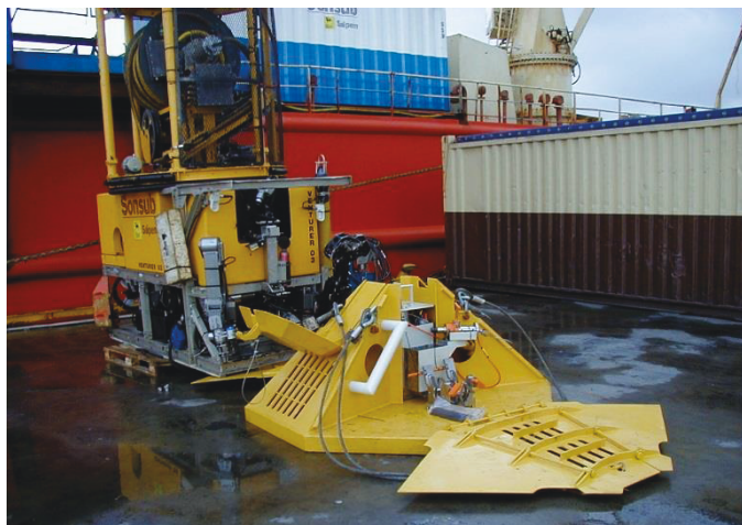
Fig. 1. ROV trial to verify operation and access
