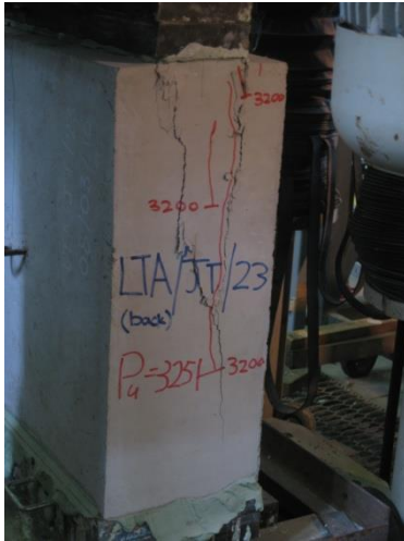
Figure 6. Full scale tests of segment joints under concentrated compression loading to simulate the hoop thrust at segment joints
