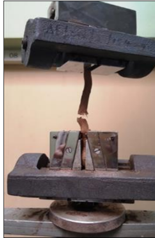
Figure 5.27 Root tensile strength testing using Dynamometer
