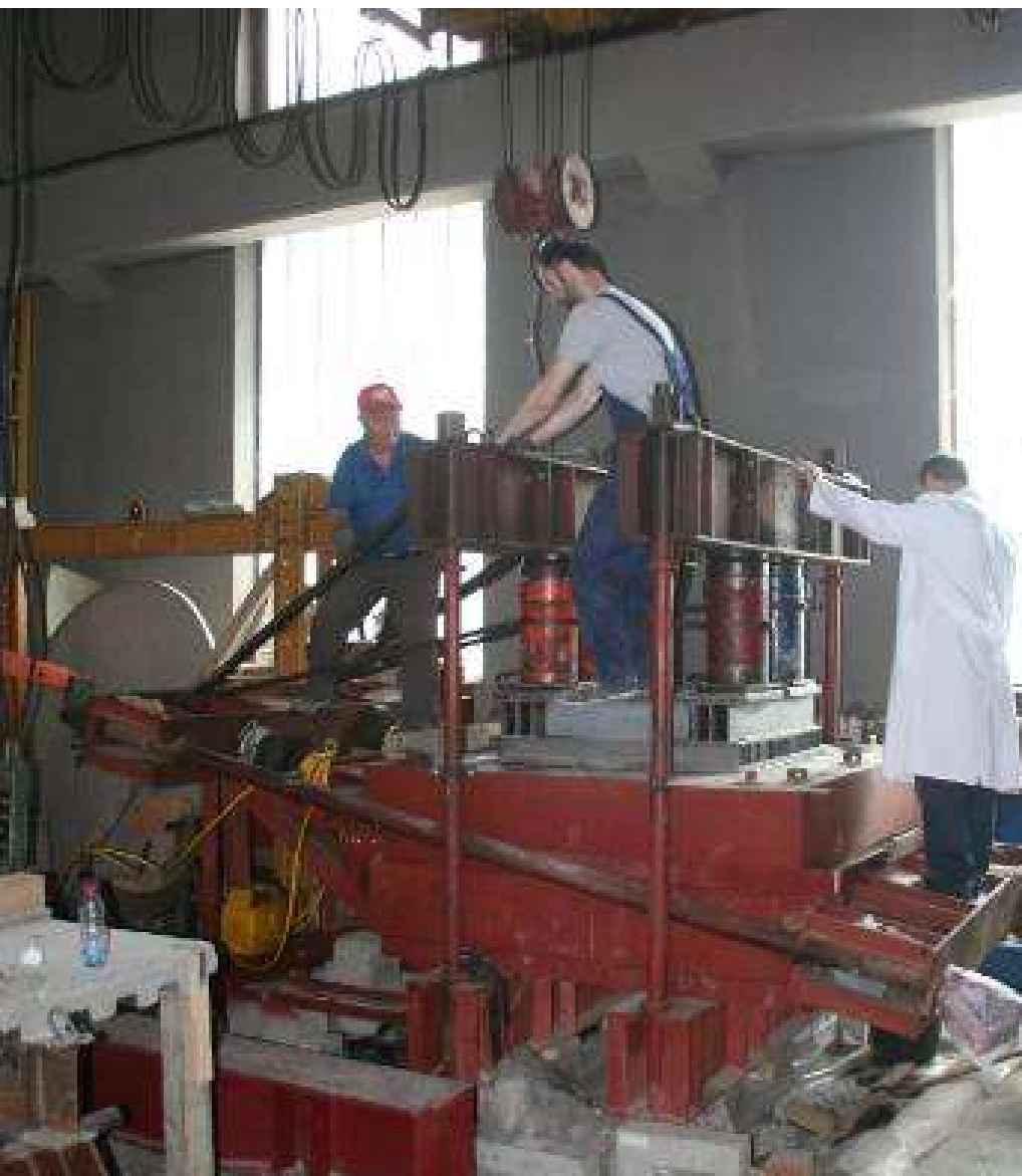
➤ Large scale direct shear 1,0x1,0x0,6 m
